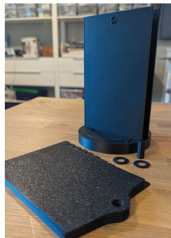
Fig. 3.31. Final stand and cards made with PLA filament. Image created by author.
