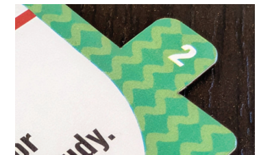
Fig. 3.23. Laser cutting the tabs created inconsistent alignment results. Image created by author.
